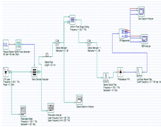
Fig 5 Simulation model (Uniform FBG)
