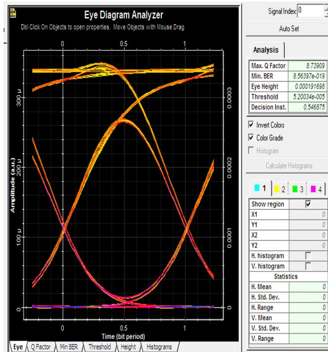
Fig8 Eye Diagram of FBG for Iteration 3
