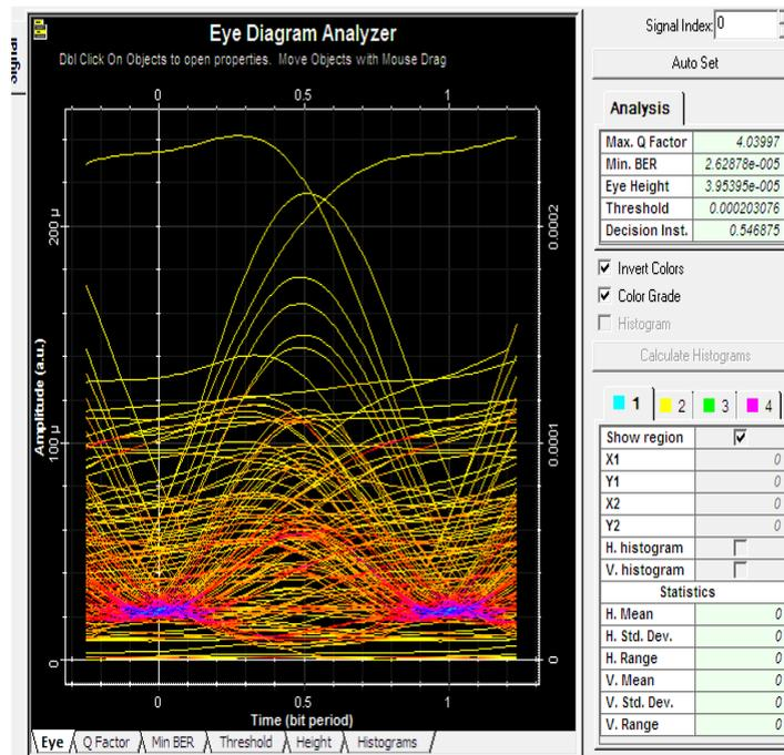
Fig6 Eye Diagram of FBG for Iteration 1
