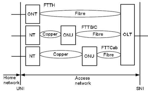
Fig 2 FTTx network Architecture
